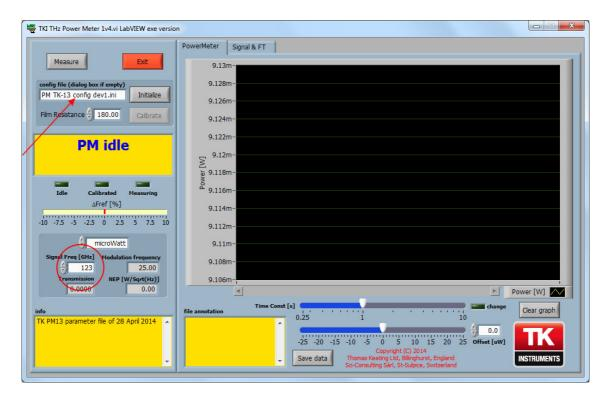
Figure 2.4: Support software main window. The arrow indicates the location of the configuration file name. The signal frequency input is circled.
