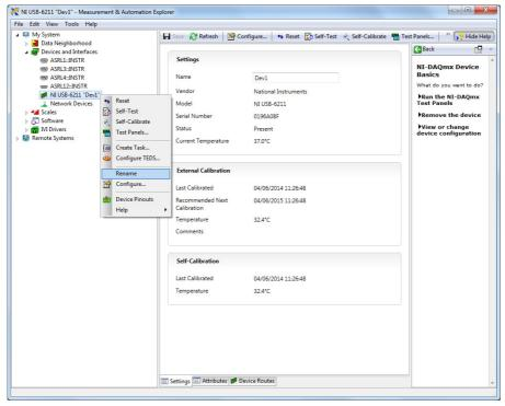
Figure 2.2: Top: NI-DAQ Measurement & Automation Explorer. Bottom: NI MAX application. Both show menu options to rename a device and to perform a self test.
