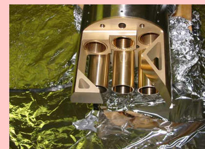
ECE oblique antenna, built from a single aluminum piece together with the terminal part of the waveguides. Courtesy Thomas Keating Ltd.
