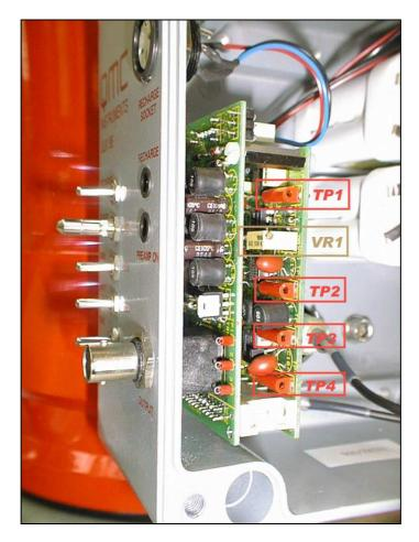
**Photo 5.3**. View of the switchboard and amplifier circuit board identifying the voltage test points and multi turn potentiometer
