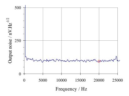
**Fig. 5.1b.** Typical preamplifier input shorted noise spectra at higher frequencies Amplifier gain = x100. Noise at  $20kHz = 1.0nV.Hz^{-1/2}$
