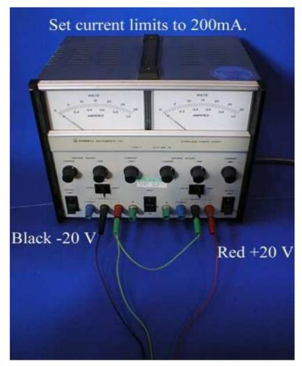
**Photo 5.2.** Power supply connections
