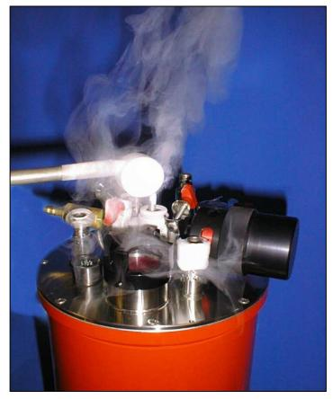
Photo 4.2. Helium gas exhaust during fill
