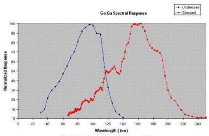
Figure 2 Spectral Response for Stressed and Unstressed Ge-Ga
