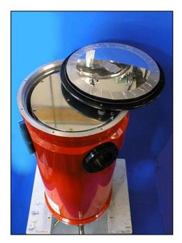
**Photo 1.4.** Liquid nitrogen base-plate in position
