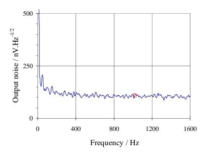
**Fig. 5.1a.** Typical preamplifier input shorted noise spectra at low frequencies Amplifier gain = x100. Noise at  $1kHz = 1.0nV.Hz^{-1/2}$
