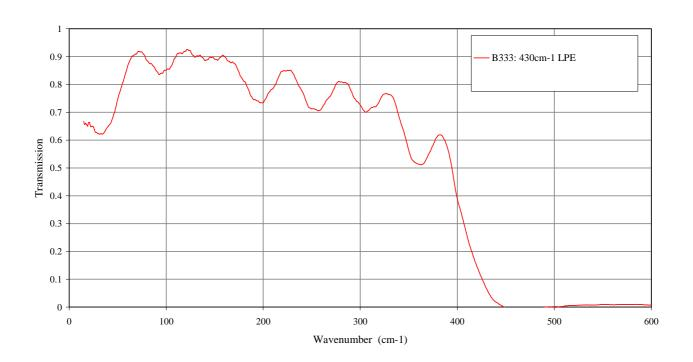
Fig C.1. Transmission spectrum for the type QMMF 430cm<sup>-1</sup> low pass filter
