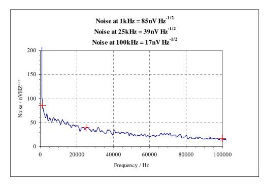
Fig. 6.2. System output noise spectrum
