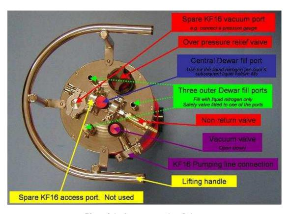
Photo 2.1. Cryostat top-plate fittings
