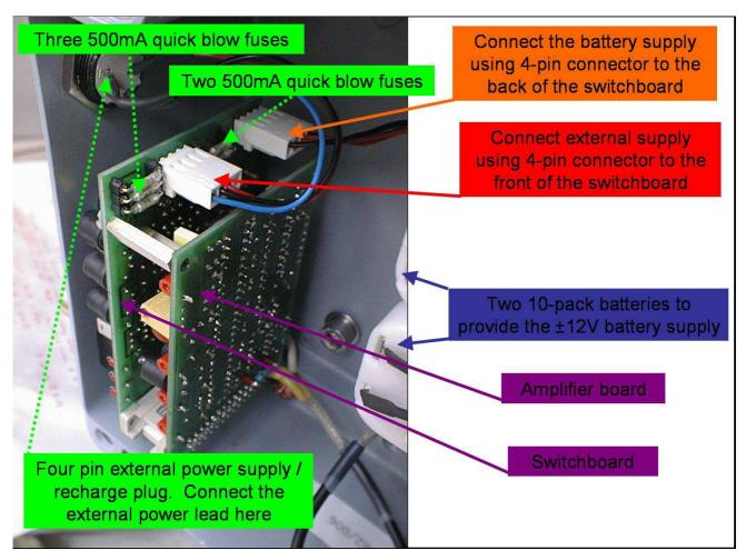
**Photo 5.1b.** Connecting the batteries
