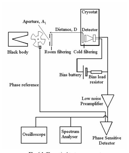
Fig. 6.1. The optical test arrangement
