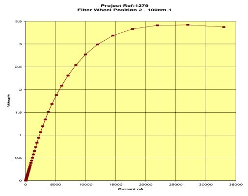
Figure 6.2b Detector VI Characteristic for filter-wheel position 2
