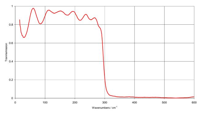
Fig. C3. Transmission spectrum for the type QMMF 300cm<sup>-1</sup> low pass filter
