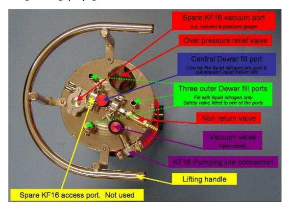
**Photo 2.1.** Cryostat top-plate fittings
