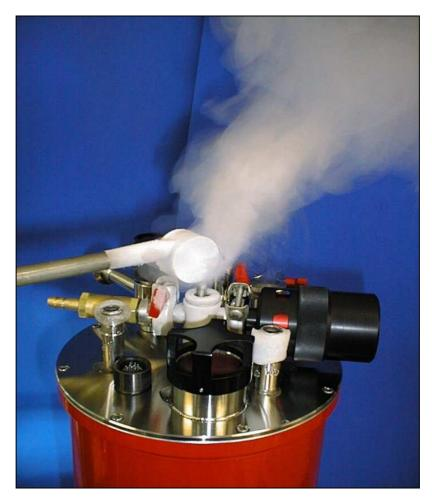
Photo 4.3. Helium plume when transfer is complete
