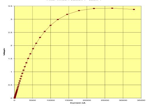
Figure 6.2a Detector VI Characteristic for filter-wheel position 1
