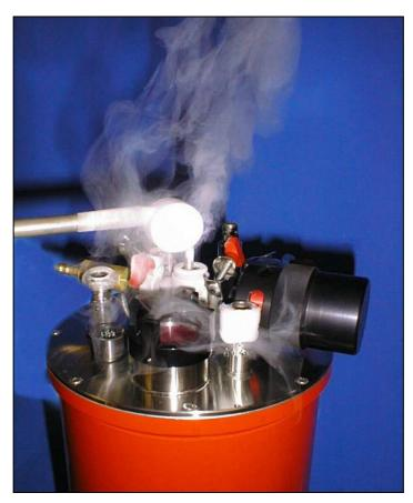
Photo 4.2. Helium gas exhaust during fill
