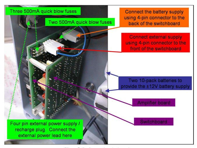
**Photo 5.1b.** Connecting the batteries
