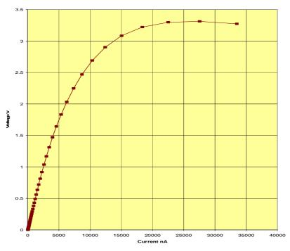
Figure 6.2c Detector VI Characteristic for filter-wheel positions 3, 4 and 5
