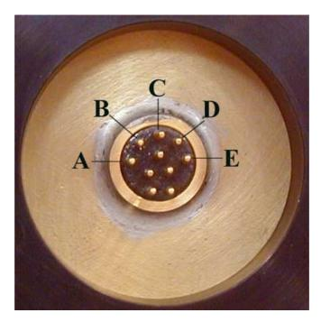
**Photo 4.4.** Electrical port pin assignments.
