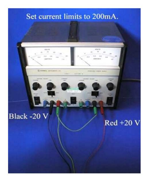
**Photo 5.2.** Power supply connections
