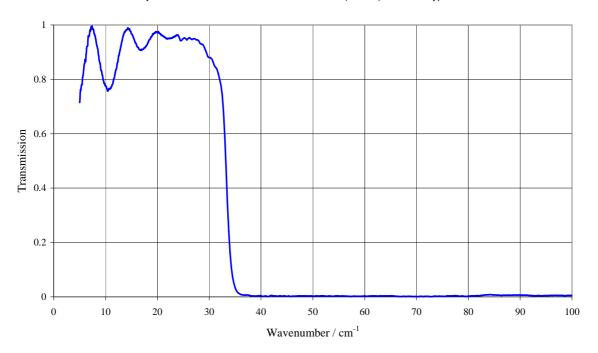
Fig. C1. Transmission spectrum for the type QMMF 33cm<sup>-1</sup> low pass filter
