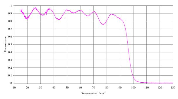
Fig. C2. Transmission spectrum for the type QMMF 100cm<sup>-1</sup> low pass filter
