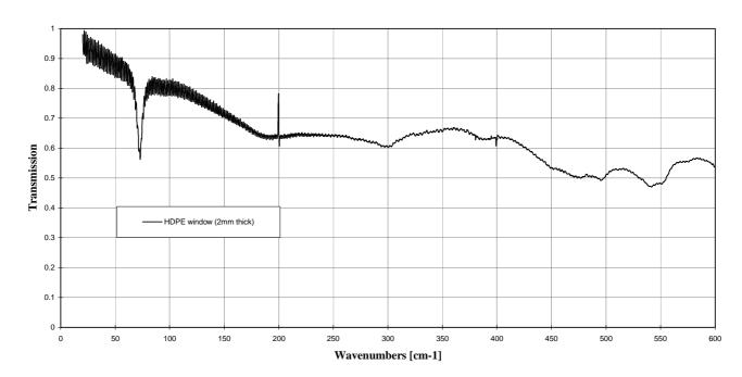
**Fig. C.4.** Measured transmission of a 2mm thick HDPE window from 20cm<sup>-1</sup> to 600cm<sup>-1</sup>. The polyethylene characteristic absorption increase is clearly seen around 73cm<sup>-1</sup>
