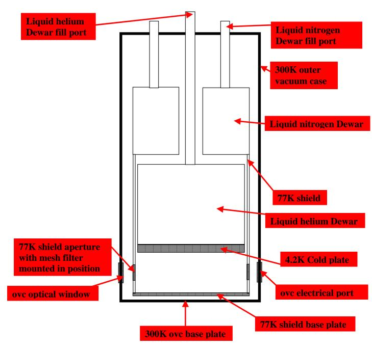
Figure 1.1. Cryostat main features. Not to scale
