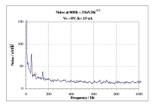
Figure 6.3. System Output Noise Spectrum
