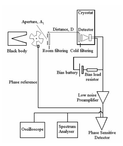
Fig. 6.1. The optical test arrangement
