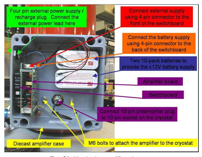
**Photo 5.1a.** Mounting the preamplifier to the cryostat
